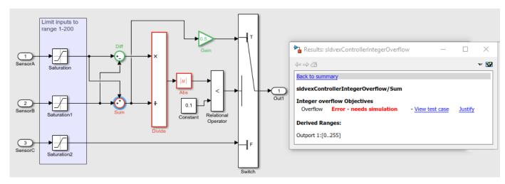
To debug the integer overflow error, click **View test case**. The harness model and the Signal Builder block open.
