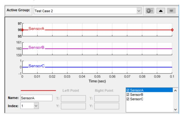
When the input value of SensorA is 96 and SensorB is 160, the Sum block output overflows. The accumulator data type of the Sum block is set to an incorrect integer value of uint8, it results in overflow errors and division by zero errors on the downstream Divide block.
